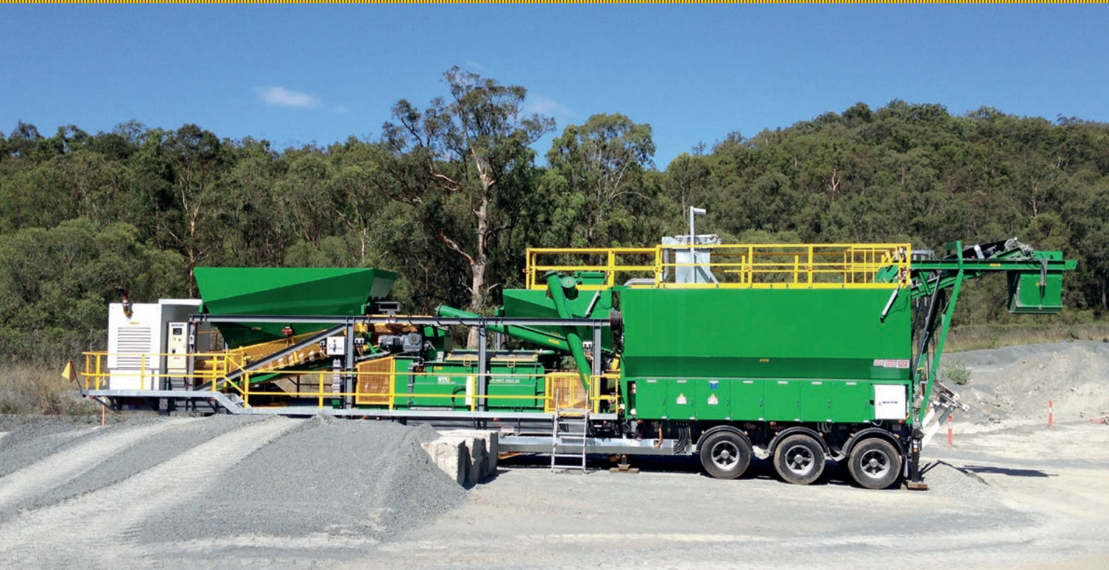
Mobile backfill paste plant
