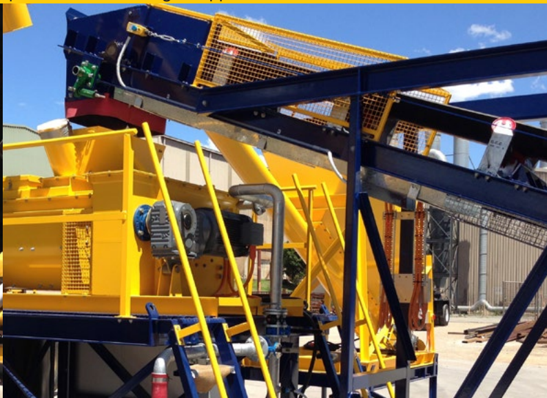
Loss of weight hopper
