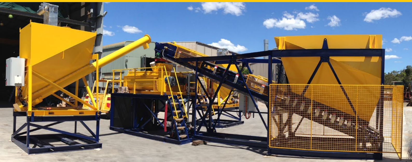
Transportable mortar and paste plant with loss of weight hopper
