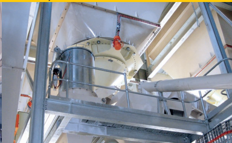
Cement screw conveyor feeding a planetary mixer with crushed glass, sand and various powdered material
