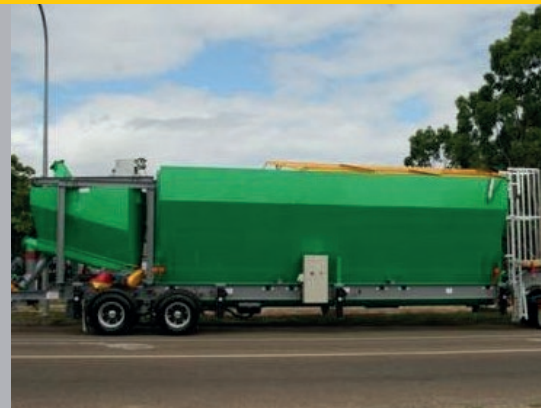
Side view configured for transport with lockable motor control centre
