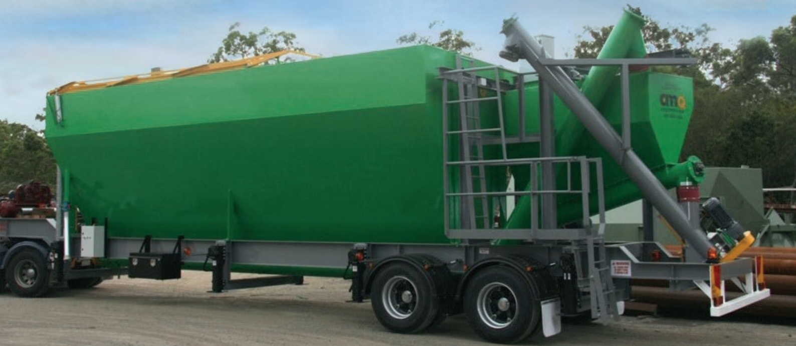
Mobile cement silo and hopper
