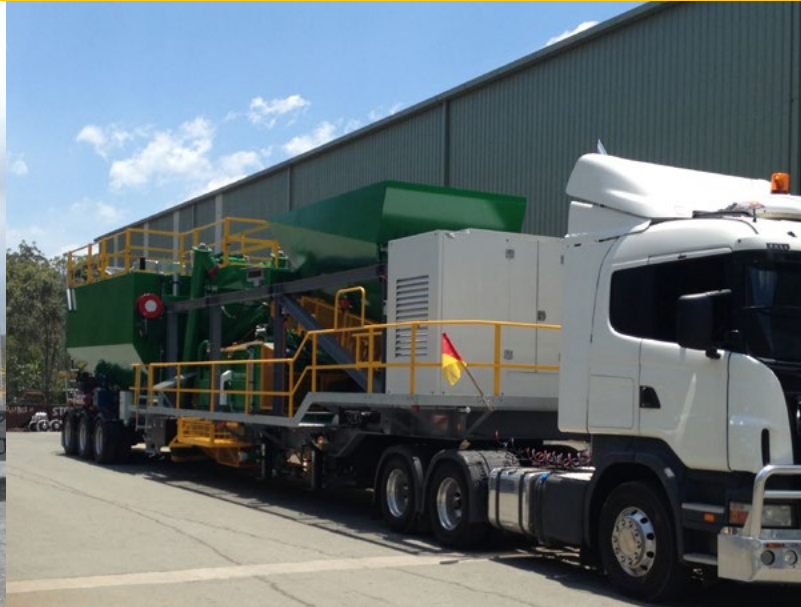
Mobile blending plant ready for transport
