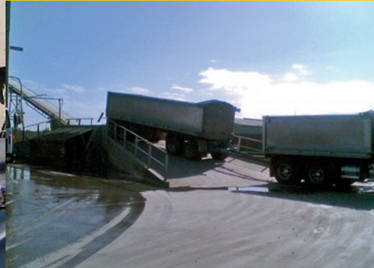
Typical low weight truck unloader plant
