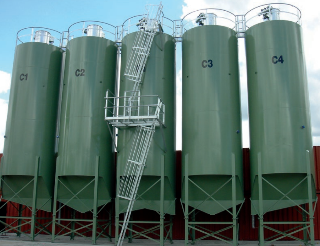
80T cement storage silos. Centre silo features dual outlet
