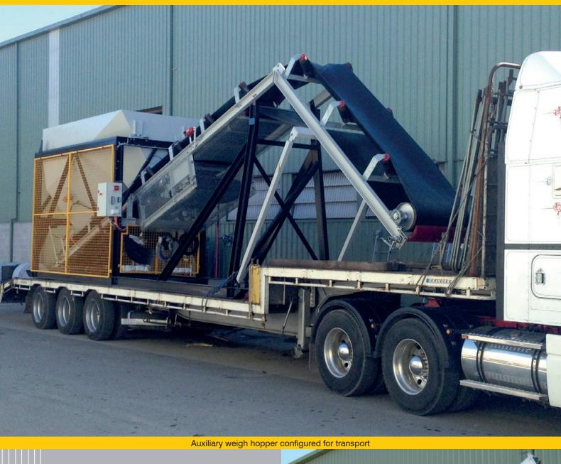
CMQ's free-standing cement weigh hopper with fork lift tyne slots is mounted on shear beam load cells on a skid base support frame (split for transport), complete with discharge auger and digital weight indicator.
