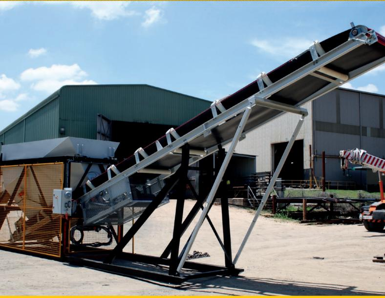
Auxiliary weigh hopper in working position
