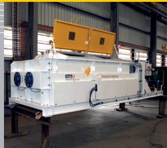
Twin shaft continuous mixer / pugmill
