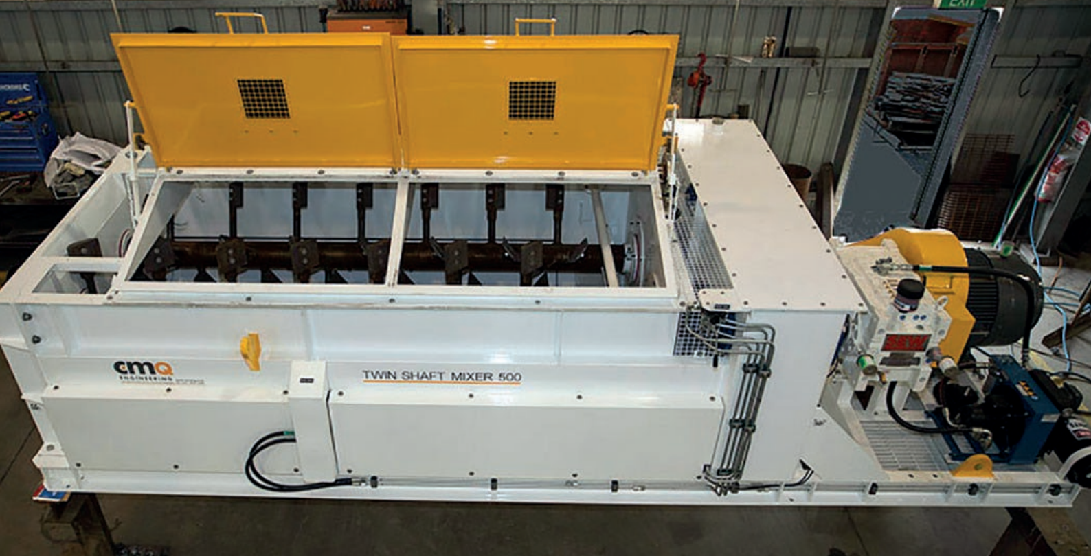
Twin shaft continuous mixer / pugmill
