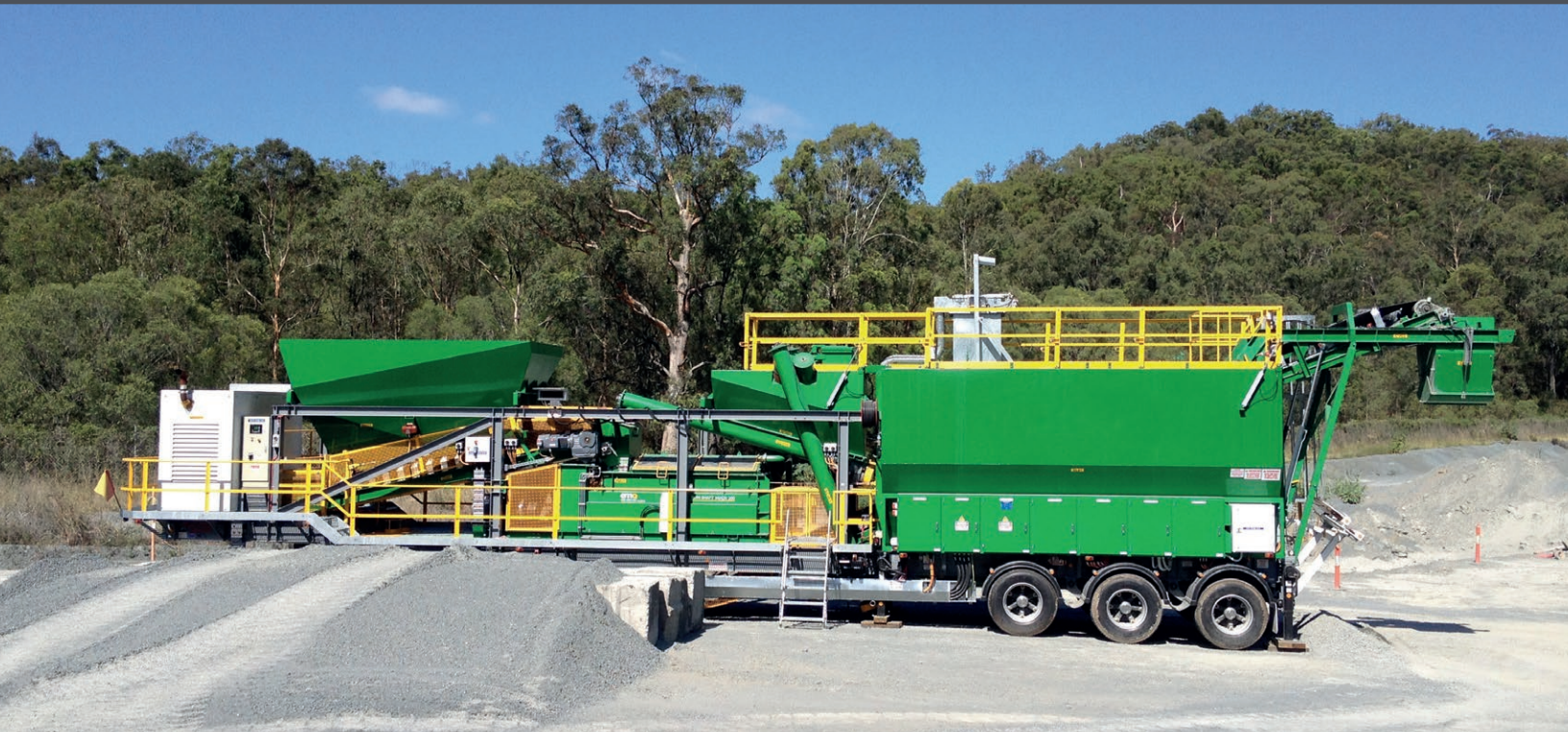
Mobile backfill paste plant
