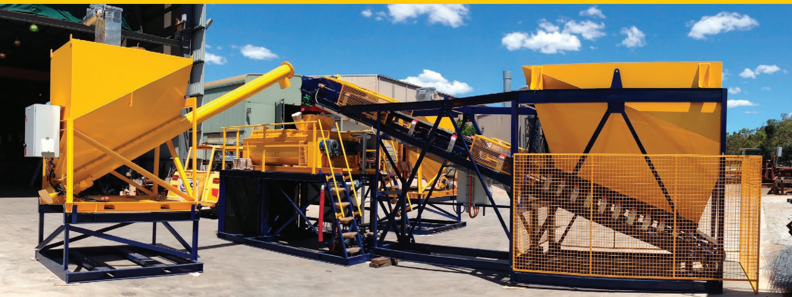
Transportable mortar and paste plant with loss of weight cement hopper and aggregate feed hopper with belt weigher conveyor
